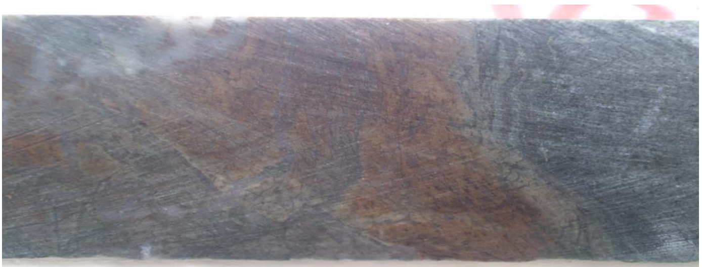
BRC111D (131.1-131.25m). Sheared Basalt. Characterised by silica-flooding and pinky cherty material, sulphides and carbonate. Assay value 131-132m - 9.69 g/t Au
